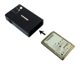
4. Make sure that the SATA drives are seated correctly on the SATA connectors of the enclosure.
